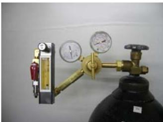
After connecting the BK assembly to the compressed breathing air source to be analyzed, the breathing air is passed through each detector tube at a specific pressure, flow rate and time interval. Each detector tube is made with high purity reagents that absorb and react with the target component. The reaction causes a colorimetric stain whose length is proportional to the component's concentration. The actual concentration is read directly from the measurement scale printed on the detector tube.
